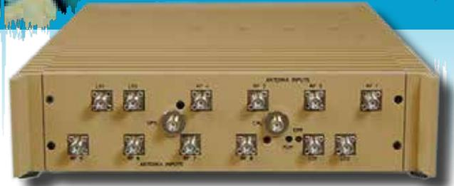
The unit includes an FPGA-based digital processor board that receives 8 channels of wideband ADC data, performs narrowband filter and decimation, forms time-stamped digital IF data packets, and transmits streaming data over the two 10 Gigabit Ethernet output ports. The dual 10 Gigabit Ethernet output ports support full bandwidth (8 x 40 MHz) data streaming. The unit is powered via an external +12 VDC power supply and controlled via a 10/100 Ethernet interface.
